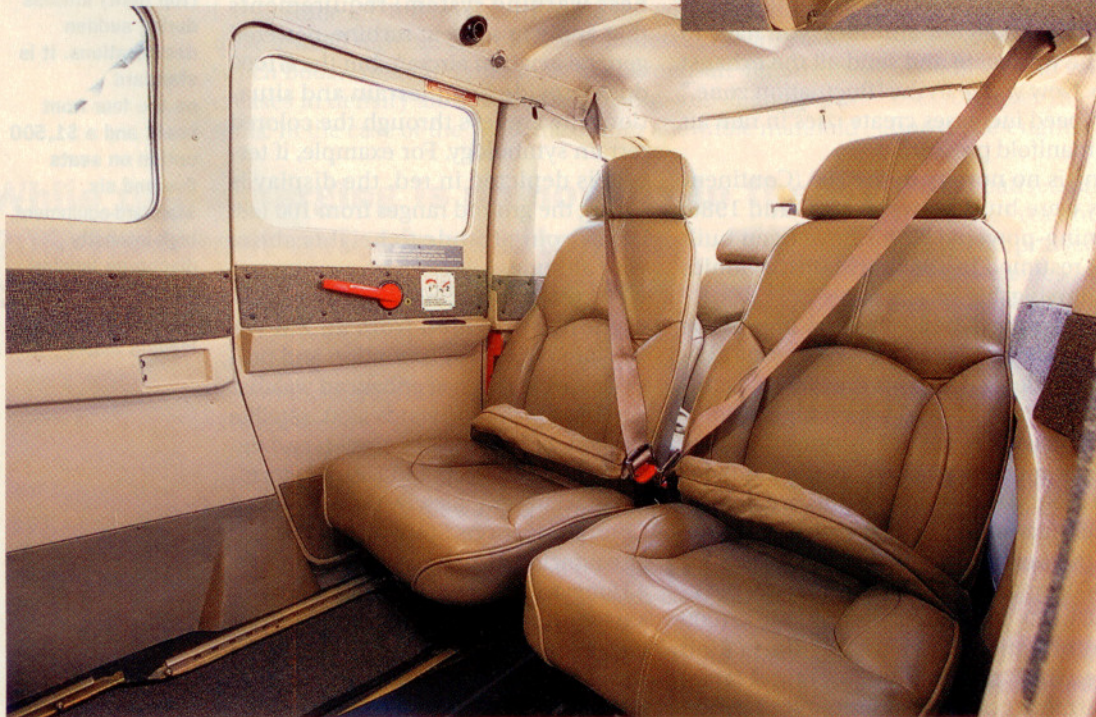
Rear dual doors open wide to let in cargo and/or passengers. Six leather seats and a built-in oxygen system are standard in T206s.
